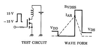
$$\begin{aligned} &RG = 25~\Omega \\ &V_{DD} = 90~V,~L = 17.4~mH \end{aligned} \quad E_{AS} = \frac{1}{2} \cdot L \cdot I^2 \cdot \left( \frac{B_{VDSS}}{B_{VDSS} - V_{DD}} \right)$$
