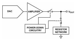
Figure 49. Output Stage During Power-Down
