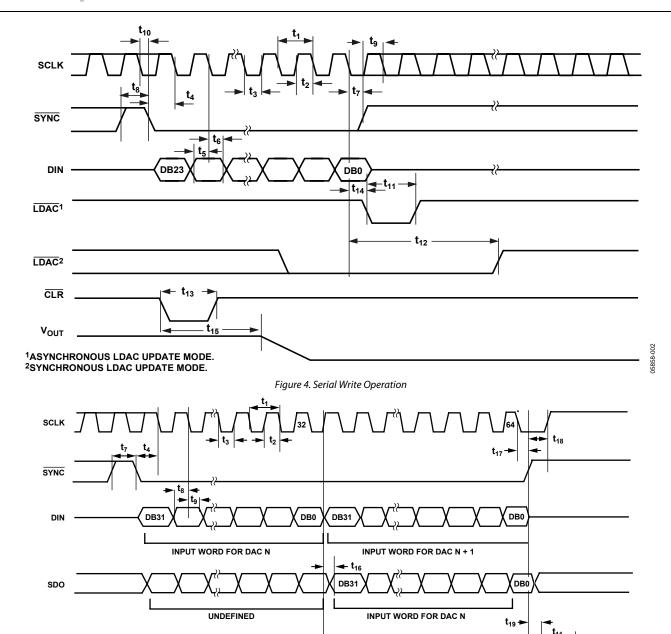
Figure 5. Daisy-Chain Timing Diagram
