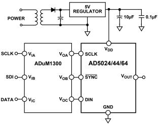
Figure 56. AD5024/44/64 with a Galvanically Isolated Interface
