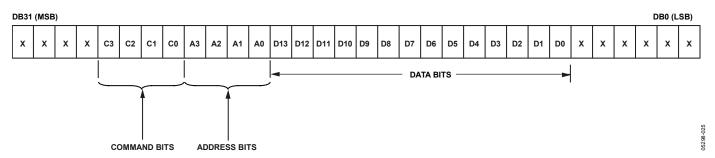
Figure 46. AD5044 Input Register Content
