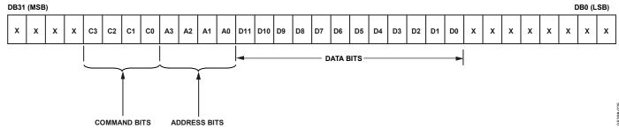
Figure 47. AD5024 Input Register Content
