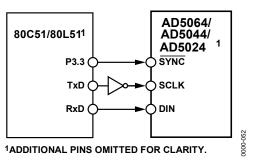
Figure 52. AD5024/44/64 to 80C512/80L51 Interface
