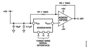
Figure 55. Bipolar Operation with the AD5024/44/64
