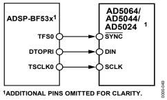
Figure 50. AD5024/44/64 to Blackfin ADSP-BF53X Interface
