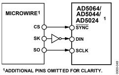
Figure 53. AD5024/44/64 to MICROWIRE Interface
