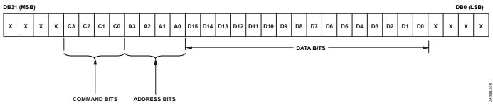
Figure 45. AD5064 Input Register Content
