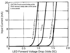
Figure 6. Input Characteristics (Current Controlled)
