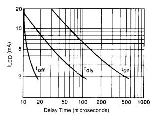
Figure 7. Typical Delay Times
