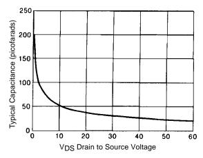
Figure 9. Typical Output Capacitance
