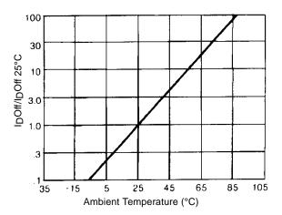
Figure 5. Normalized Off-State Leakage
