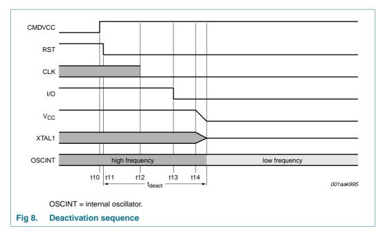
**Remark:** The value of period T is 64 times the period interval of the internal oscillator (i.e.  $\pm$  25  $\mu$ s).
