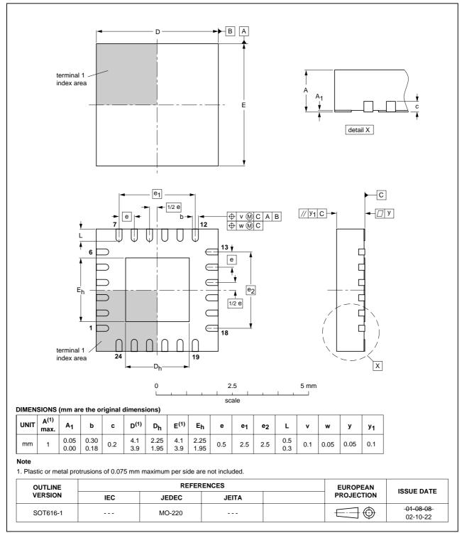
HVQFN24: plastic thermal enhanced very thin quad flat package; no leads; 24 terminals; body 4 x 4 x 0.85 mm
