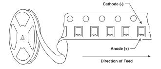
**Tape and Reel Specifications**: All case codes are available on plastic embossed tape per EIA-481-1. Tape reeling per IEC 286-3 is also available. Standard reel diameter is 13" [330mm]. 7" [178mm] reels are available.
