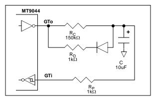
Figure 12 - Unsymmetrical Guard Time Circuit
