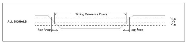
Figure 18 - Timing Parameter Measurement Voltage Levels
