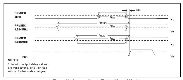
Figure 19 - Input to Output Timing (Normal Mode)
