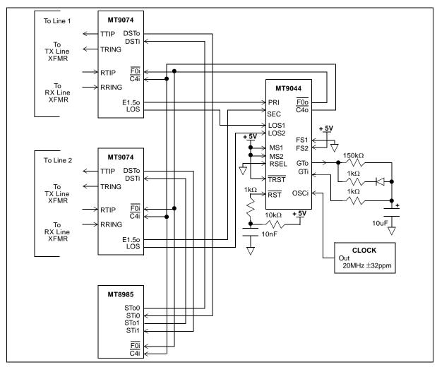
Figure 15 - Dual T1 Reference Sources with MT9044 in 1.544MHz Automatic Control
