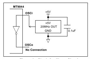
Figure 9 - Clock Oscillator Circuit
