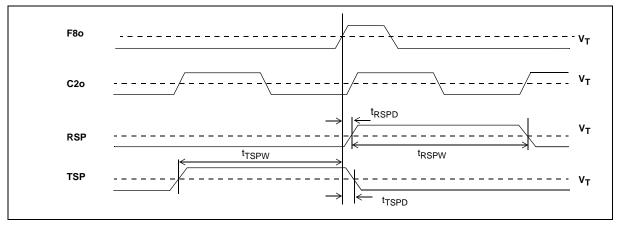
Figure 21 - Output Timing 2
