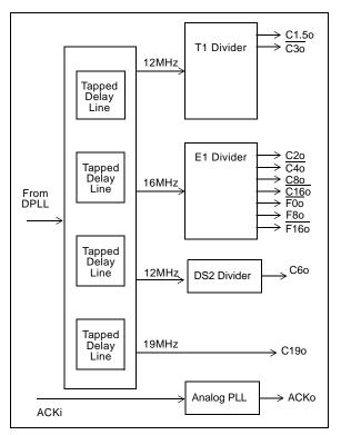
Figure 5 - Output Interface Circuit Block
