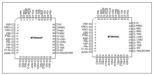
Figure 2 - Pin Connections
