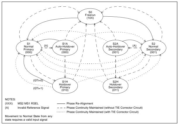
Figure 7 - Manual Control State Diagram
