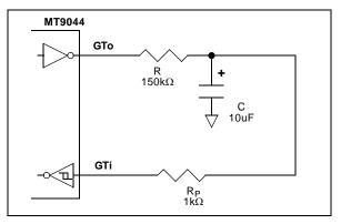
Figure 11 - Symmetrical Guard Time Circuit
