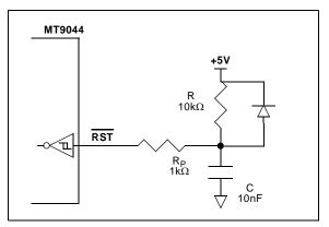
Figure 14 - Power-Up Reset Circuit
