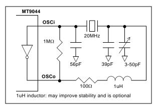
Figure 10 - Crystal Oscillator Circuit
