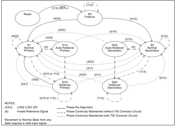
Figure 8 - Automatic Control State Diagram
