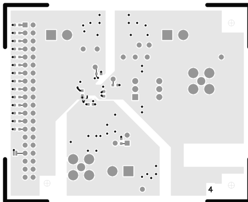
Figure 31. LFCSP Evaluation Board Layout—Secondary Side
