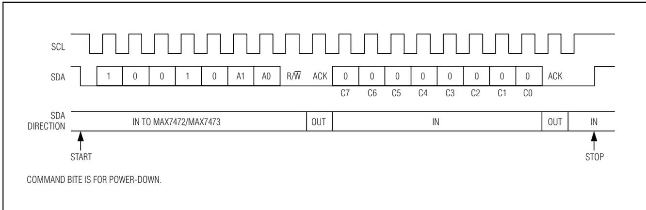
Figure 7. Write Sequence for a Command Byte
