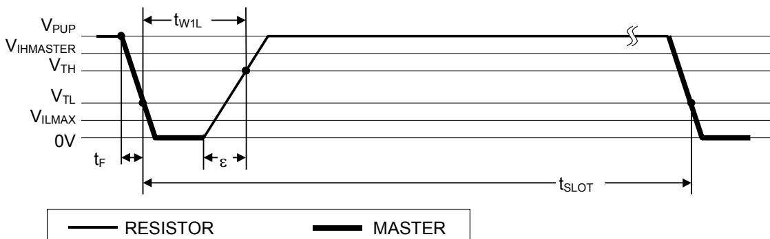
Figure 11. READ/WRITE TIMING DIAGRAM
