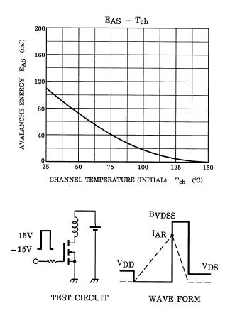
$$\begin{array}{l} \mathrm{R_{G}=25\ \Omega}\\ \mathrm{V_{DD}=50\ V,\ L=2.47\ mH} \end{array} \qquad \mathrm{EAS}=\frac{1}{2}\cdot\mathrm{L}\cdot\mathrm{I}^{2}\cdot\left(\frac{\mathrm{BVDSS}}{\mathrm{BVDSS}-\mathrm{VDD}}\right) \end{array}$$
