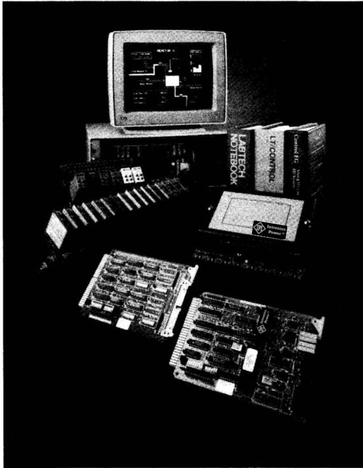
Analog Devices RTI-1265/1266/1267 Series STD Bus I/O Boards Are Compatible with Signal Conditioning Panels and IBM PC Application Software.
