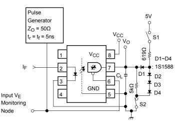
C<sub>L</sub> is approximately 15pF which includes probe and stray wiring capacitance.
