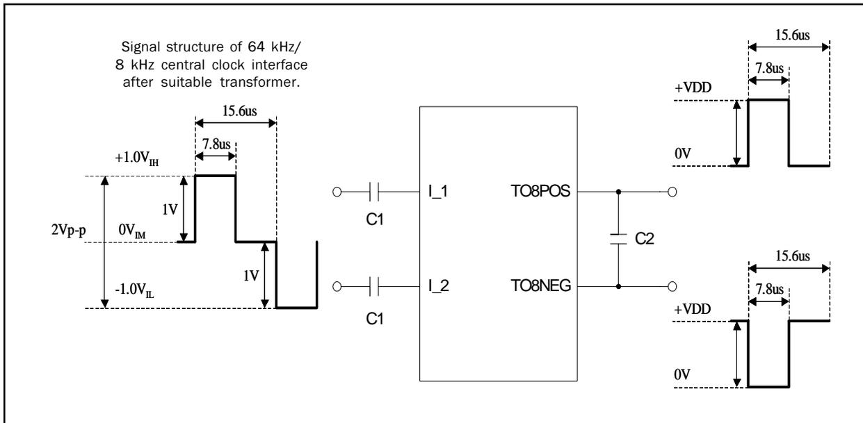
**Figure 16. Recommended Line Termination for AMI Output/Output Ports**
