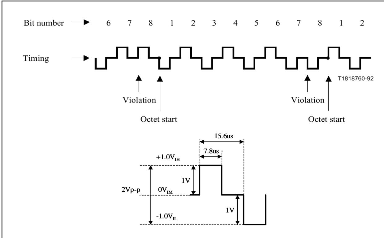
**Figure 15. AMI Input and Output Signal Levels**
