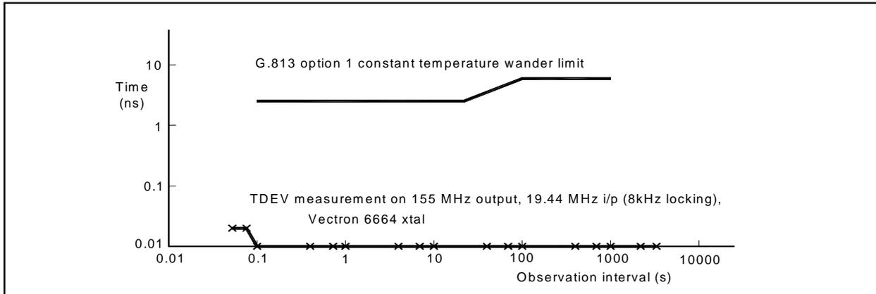
**Figure 8. Phase error accumulation of  $T_{OUT0}$  output port in Holdover mode**
