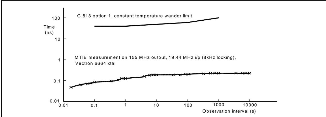
**Figure 7. Time Deviation of  $T_{OUT0}$  output port**
