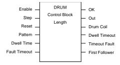
Power flow to the Enable input causes the Drum Sequencer to copy the content of the selected reference pattern to the Out reference.
