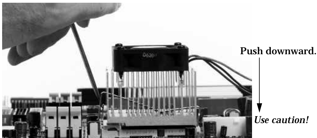
Figure 15. Pushing the Heatsink Clip Down
