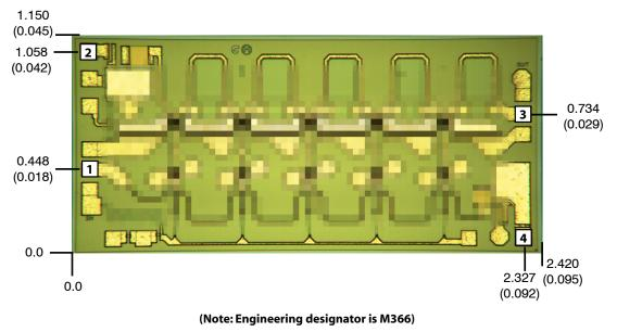
Units: millimeters (inches) Bond pad dimensions are shown to center of bond pad. Thickness: 0.110 +/- 0.010 (0.0043 +/- 0.0004), Backside is ground, Bond Pad/Backside Metallization: Gold All DC and RF Bond Pads are ~0.080 x 0.080 (0.003 x 0.003). Bond pad centers are approximately 0.109 (0.004) from the edge of the chip. Dicing tolerance: +/- 0.005 (+/- 0.0002). Approximate weight: 1.73 mg.
