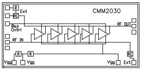
controlled to maintain correct drain current and thus drain voltage. The typical gate voltage needed to do this is 0.5V. Typically the gate is protected with Silicon diodes to limit the applied voltage. Also, make sure to sequence the applied voltage to ensure negative gate bias is available before applying the positive drain supply.
