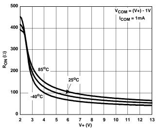
FIGURE 9. ON RESISTANCE vs SUPPLY VOLTAGE
