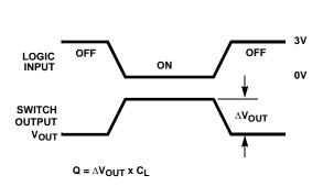
FIGURE 2A. MEASUREMENT POINTS
