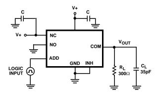
Repeat test for other switches. C<sub>L</sub> includes fixture and stray capacitance.
