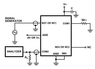
FIGURE 6. CROSSTALK TEST CIRCUIT
