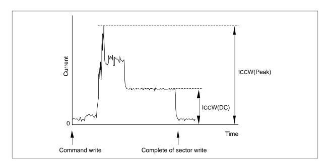
AC Characteristics (Ta = 0 to +60°C,  $V_{CC}$  = 5 V  $\pm$  10%, 3.3 V  $\pm$  5%)
