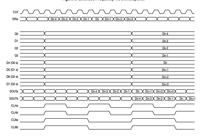
Figure 9. Timing Diagram A. 1:8 Serial to Parallel Conversion
