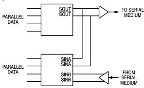
Figure 5. Loopback Test Architecture
