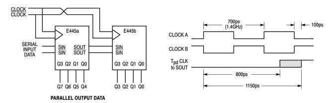
Figure 8. Extended Frequency 1:8 Demultiplexer
