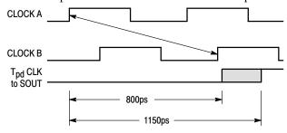
Figure 7. Cascade Frequency Limitation
