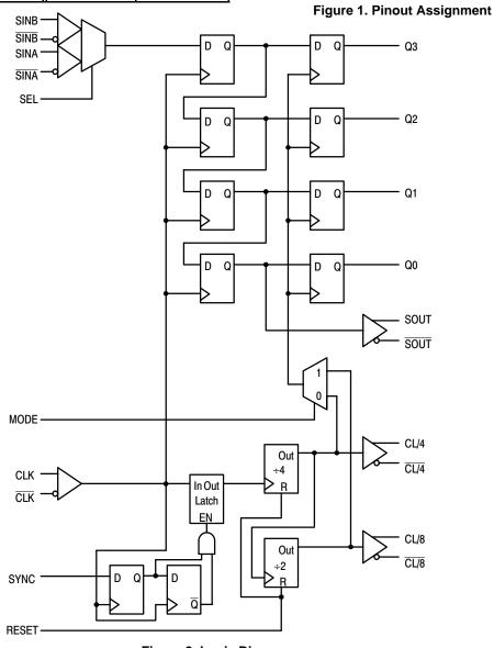
Figure 2. Logic Diagram
