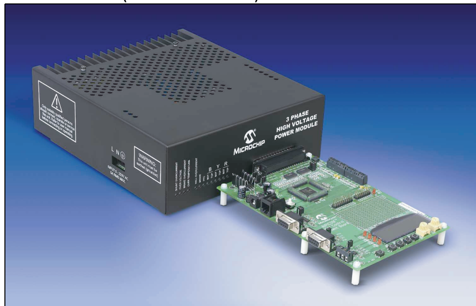
FIGURE 1-1: POWER MODULE WITH ATTACHED DEVELOPMENT BOARD (SOLD SEPARATELY)
