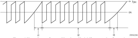
Figure 1 Motor Output Current Waveform Model (Commutation Current)
