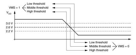
Figure 13. External Input Voltage Supervisor
