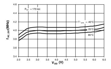
Figure 71. System Clock versus V<sub>DD</sub>
