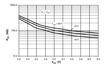
Figure 79. Strong Pull-down Resistor versus V<sub>DD</sub>
