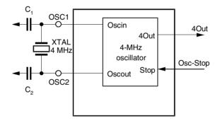
Figure 19. Ceramic Resonator
