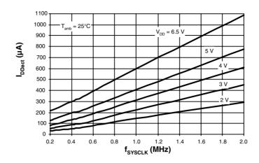
Figure 64. Power-down Supply Current versus Frequency
