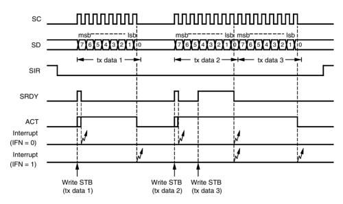
Figure 46. Example of 8-bit Synchronous Receive Operation
