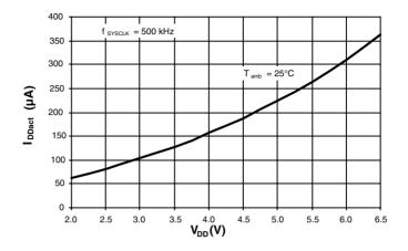
Figure 67. Power-down Supply Current versus V<sub>DD</sub>
