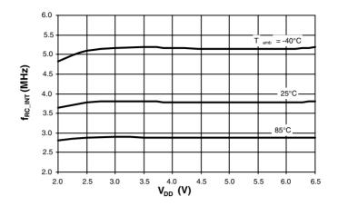
Figure 70. External RC Frequency versus  $V_{DD}$
