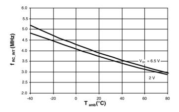
Figure 73. External RC Frequency versus T<sub>amb</sub>
