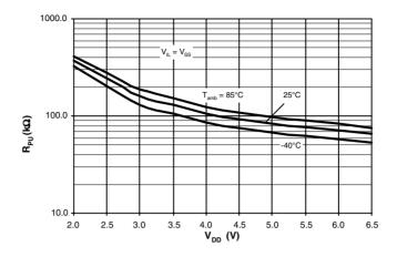
Figure 76. Strong Pull-up Resistor versus V<sub>DD</sub>
