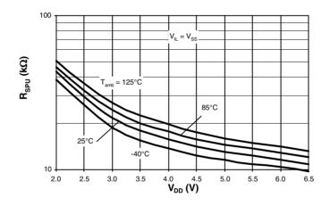
Figure 101. Strong Pull-down Resistor versus  $V_{\rm DD}$
