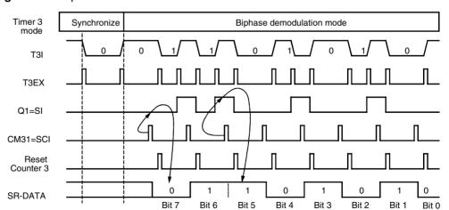
Figure 77. Bi-phase Demodulation
