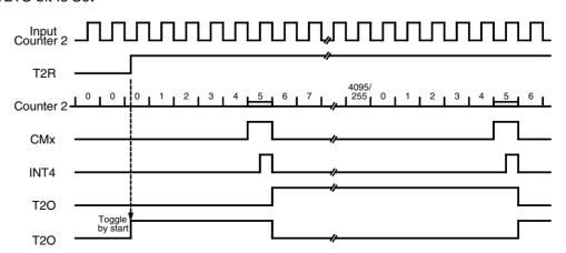
Toggle Mode C: A Timer 2 compare match toggles the output flip-flop (M2) -> T2O
