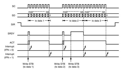
Figure 60. Example of an 8-bit Synchronous Receive Operation
