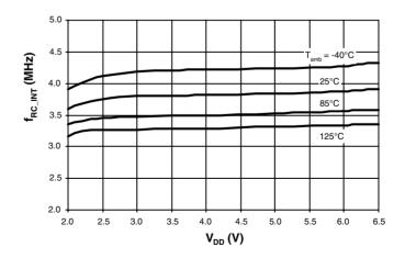
Figure 93. Internal RC Frequency versus  $T_{amb}$
