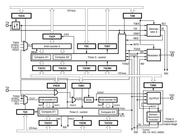
Combination Mode 10: Frequency Measurement or Event Counter with Time Gate Timer 2 mode 1/2: 12-bit compare counter/8-bit compare counter and
