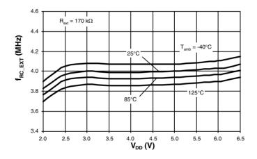
Figure 95. External RC Frequency versus T<sub>amb</sub>
