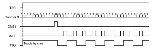
Timer 3 – Mode 2: Timer/Counter, External Trigger Restart and External Capture (with T3I Input)
