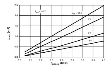
Figure 88. Active Supply Current versus  $V_{\text{DD}}$
