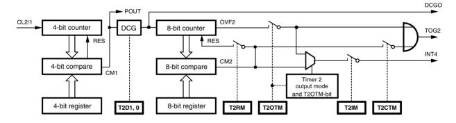
The 4-bit stage is used as programmable prescaler for the 8-bit counter stage. In this mode, a duty cycle stage is also available. This stage can be used as an additional 2-bit prescaler or for generating duty cycles of 25%, 33% and 50%. The 4-bit compare output (CM1) supplies the clock output (POUT) with clocks.
