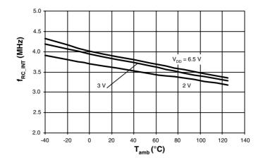
Figure 94. External RC Frequency versus  $V_{\rm DD}$
