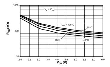
Figure 99. Pull-down Resistor versus  $V_{\rm DD}$
