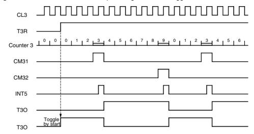
Figure 47. Single Action of Compare Register 1
