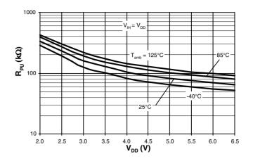
Figure 100. Strong Pull-up Resistor versus  $V_{\rm DD}$
