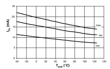
Figure 105. Output Low Current versus  $T_{amb}$ ,  $V_{DD}$  = 6.5 V,  $V_{OL}$  = 0.2 ×  $V_{DD}$
