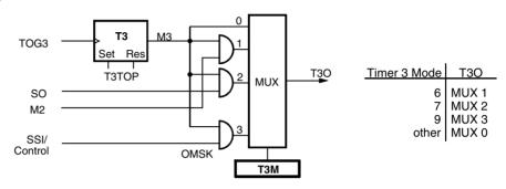
Timer 3 Demodulator for Bi-phase, Manchester and Pulse-width-modulated Signals
