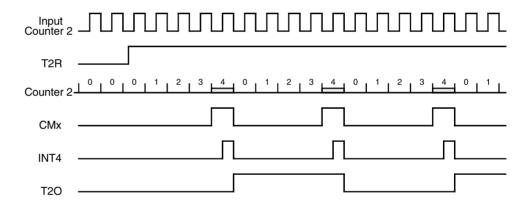
Toggle Mode B: A Timer 2 compare match toggles the output flip-flop (M2) -> T2O
