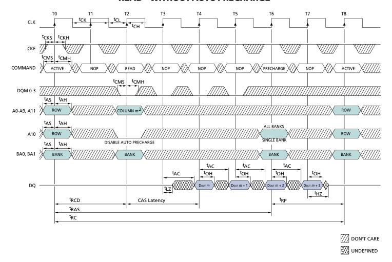
**NOTE:** 1. For this example, the burst length = 4, the CAS latency = 2, and the READ burst is followed by a "manual" PRECHARGE.
