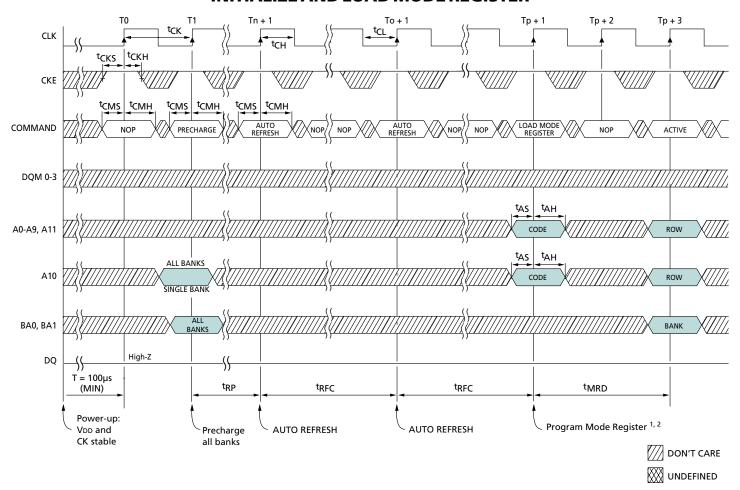
**NOTE:** 1. The Mode Register may be loaded prior to the AUTO REFRESH cycles if desired.
