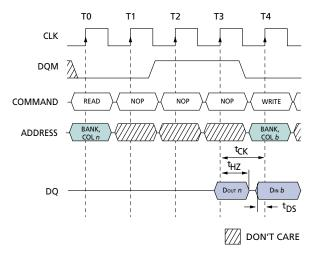
NOTE: A CAS latency of three is used for illustration. The READ command may be to any bank, and the WRITE command may be to any bank. If a burst of one is used, then DQM is not required.
