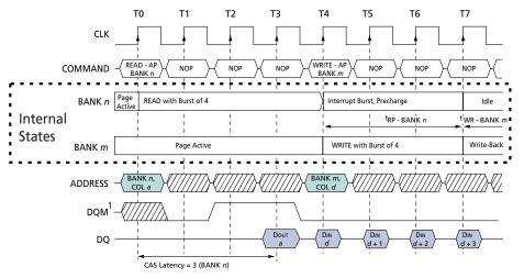
NOTE: 1. DQM is HIGH at T2 to prevent Dout-a+1 from contending with DIN-d at T4.
