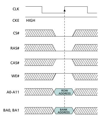
Figure 4 Example: Meeting  ${}^{t}RCD$  (MIN) When 2 <  ${}^{t}RCD$  (MIN)/ ${}^{t}CK$  - 3
