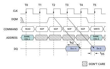
NOTE: A CAS latency of three is used for illustration. The READ command may be to any bank, and the WRITE command may be to any bank.
