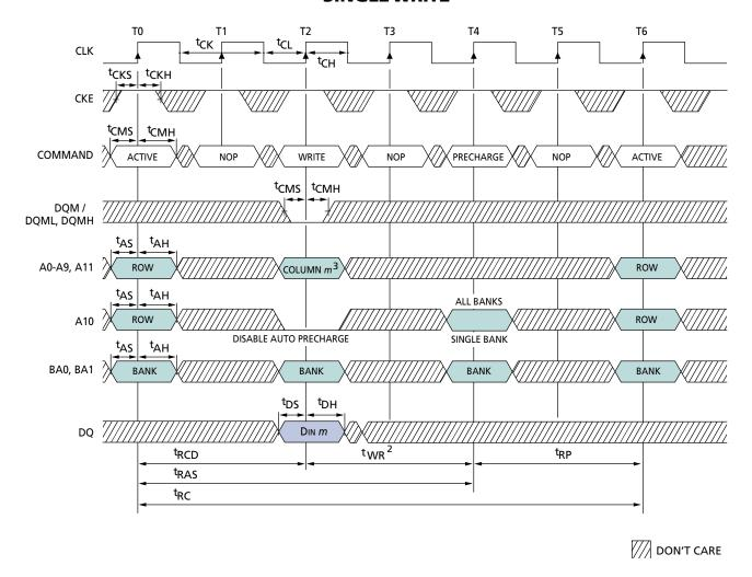
NOTE: 1. For this example, the burst length = 1, and the WRITE burst is followed by a "manual" PRECHARGE.
