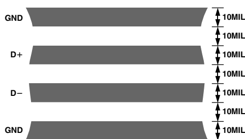
Figure 13. Arrangement of Signal Tracks
