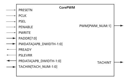
Figure 1-2 · CorePWM I/O Signal Diagram
