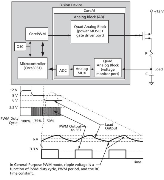
In Low-Ripple DAC mode, pulse width is effectively reduced to 1 clock cycle period, significantly reducing the ripple at the output of a low pass filter.
