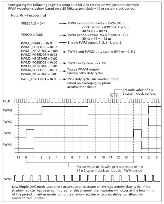
Figure 1-3 · CorePWM Waveform Generation Example
