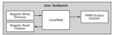
Figure 2-3 · CorePWM Verification Testbench
