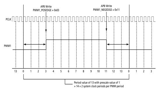
Figure 1-5 · Center-Aligned PWM Waveform Example
