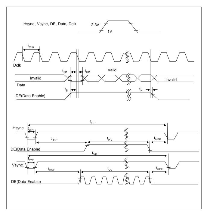
[ Figure 6 ] Signal timing waveforms
