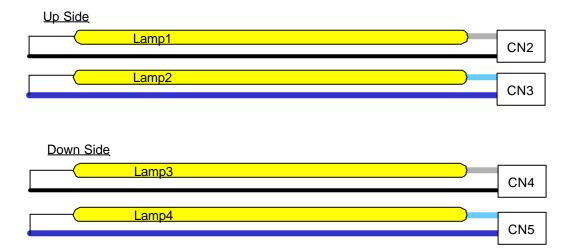
[ Figure 5 ] Backlight connector view
