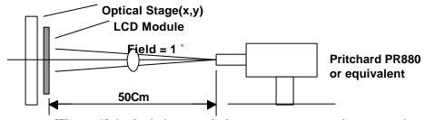
[Figure 9] Optical characteristic measurement equipment and method
