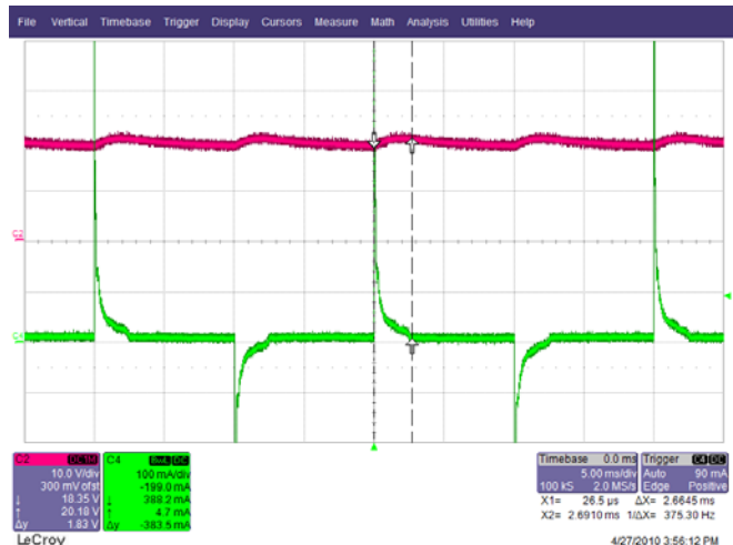
Figure 35 – 230 VAC, 49° Phase. Upper: V_{OUT} , 10 V / div. Lower: I_{IN} , 0.1 A / div., 5 ms / div.
