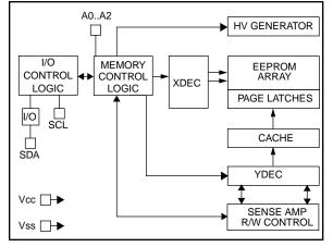
up to eight 24FC65's on the same bus for up to 512K bits contiguous EEPROM memory. The 24FC65 is available in the standard 8-pin plastic DIP and 8-pin surface mount SOIC package.
