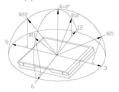
Note  $10-2: CR = \frac{\text{Luminance when Testing point is White}}{\text{Luminance when Testing point is Black}}$ (Testing configuration see 10-2)
