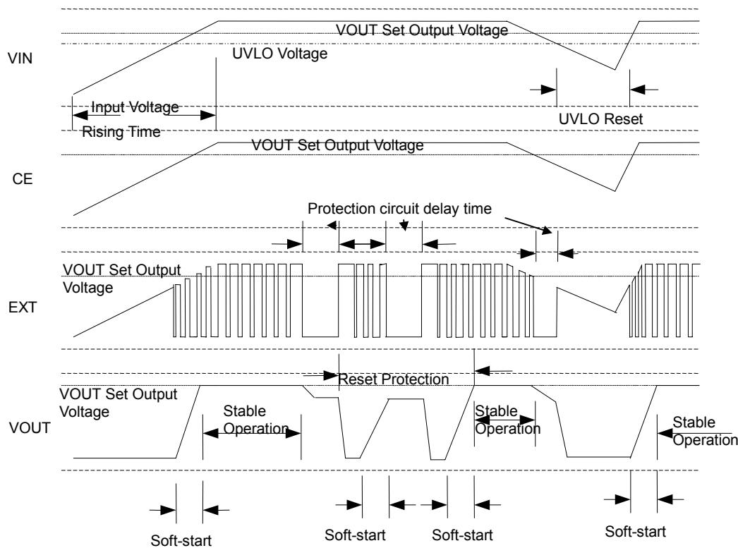
The timing chart shown above describes the changing process of input voltage rising, stable operating, operating with large current, stable operating, input voltage falling, input voltage recovering, and stable operating.
