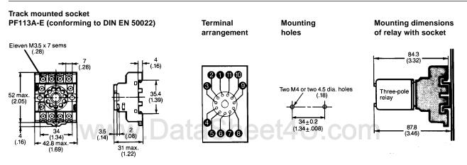
Note: Model PF113A-E can be used as a front connecting socket.
