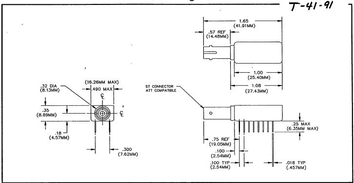
The metal housings of these modules are conductive and should be prevented from contacting circuit board traces or the sleeves of low profile screw machine sockets. A thin plastic DIP insulator (such as BIVAR, Inc. Part Number 816-030 or equivalent) is recommended.
