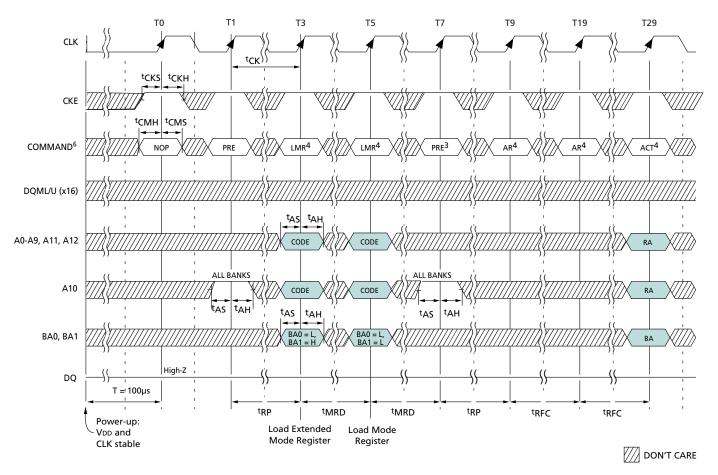
NOTE: 1. The two AUTO REFRESH commands at T9 and T19 may be applied before either LOAD MODE REGISTER (LMR) command.
