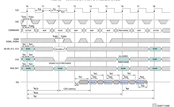
**NOTE:** 1. For this example, the burst length = 4, the CAS latency = 2, and the READ burst is followed by a "manual" PRECHARGE.
