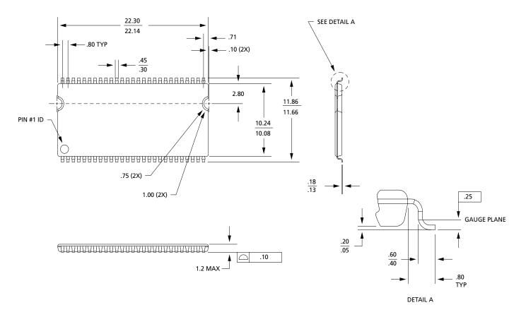
**NOTE:** 1. All dimensions in millimeters or typical where noted.
