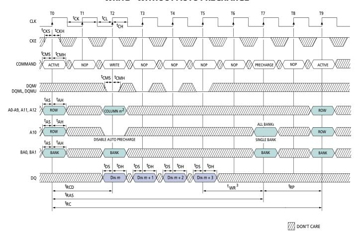
NOTE: 1. For this example, the burst length = 4, and the WRITE burst is followed by a "manual" PRECHARGE.
