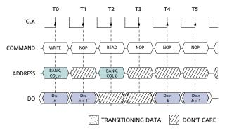
NOTE: The WRITE command may be to any bank, and the READ command may be to any bank. DQM is LOW. CAS latency = 2 for illustration.
