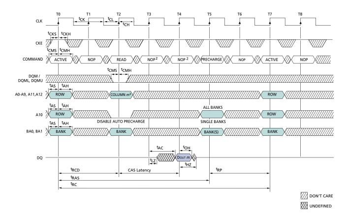
**NOTE:** 1. For this example, the burst length = 1, the CAS latency = 2, and the READ burst is followed by a "manual" PRECHARGE.
