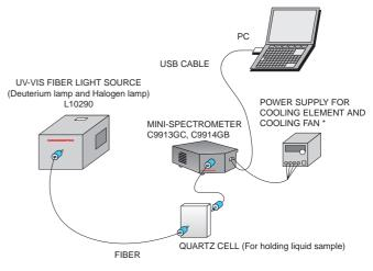
\* External power supply should be prepared by the user. C9406GC: No external power supply required (Uses USB bus power)
