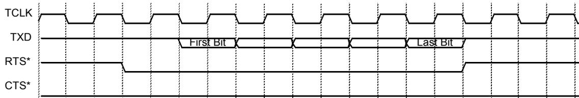
**Figure 94: Output Delay From RTS\*, Synchronous CTS\***
