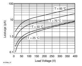
Figure 7. Leakage Current vs. Applied Voltage
