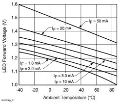
Figure 1. LED Voltage vs. Temperature
