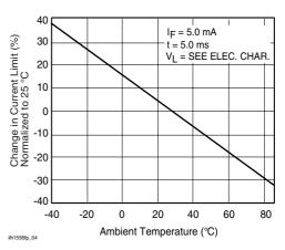
Figure 4. Current Limit vs. Temperature
