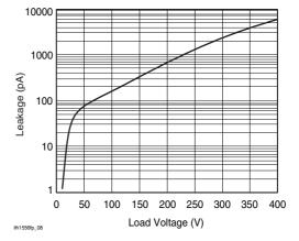
Figure 8. Leakage Current vs. Applied Voltage
