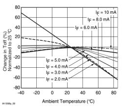
Figure 9. Turn-off Time vs. Temperature
