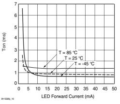
Figure 10. Turn-on Time vs. LED Current
