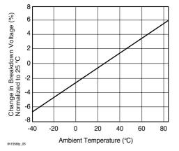
Figure 5. Switch Breakdown Voltage vs. Temperature
