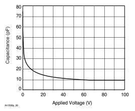
Figure 6. Switch Capacitance vs. Applied Voltage
