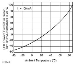
Figure 2. LED Current for Switch Turn-on vs. Temperature
