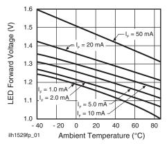
Fig. 1 - LED Voltage vs. Temperature
