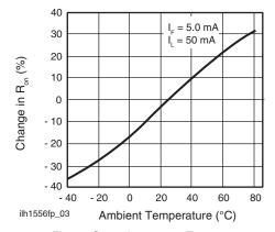
Fig. 3 - On-resistance vs. Temperature
