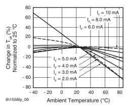
Fig. 9 - Turn-off Time vs. Temperature
