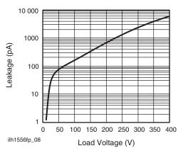
Fig. 8 - Leakage Current vs. Applied Voltage
