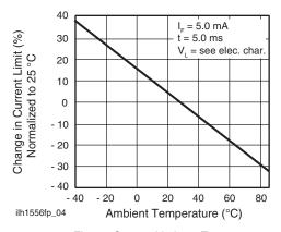
Fig. 4 - Current Limit vs. Temperature
