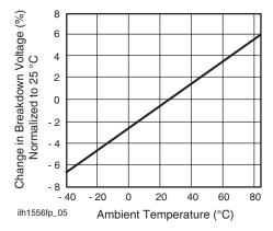
Fig. 5 - Switch Breakdown Voltage vs. Temperature
