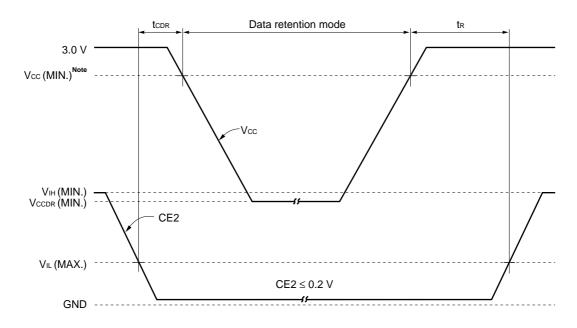
$\textbf{Note} \quad \text{B version}: 2.7 \text{ V, C version}: 2.2 \text{ V, D version}: 1.8 \text{ V}$
