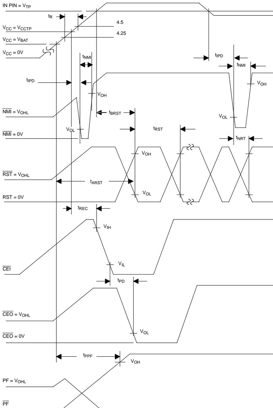
**WAKE/SLEEP CONTROL** Figure 13
