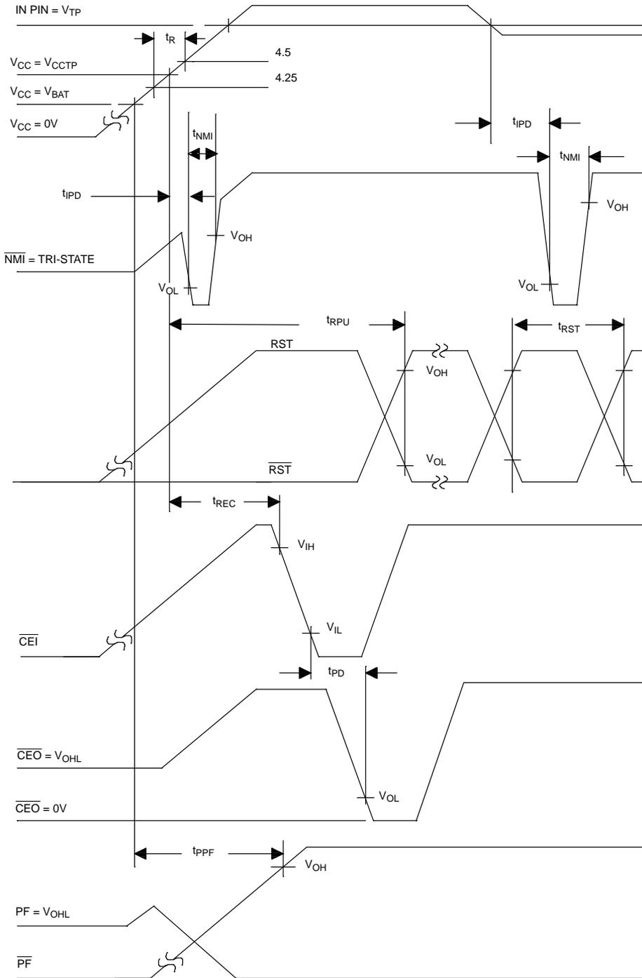
CMOS MODE POWER-UP (RC = V<sub>CC0</sub>) Figure 12
