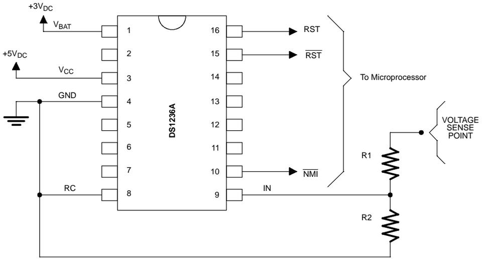
EXAMPLE 1: 5 VOLT SUPPLY, R2 = 10K OHM,  $V_{SENSE} = 4.80$  VOLTS
