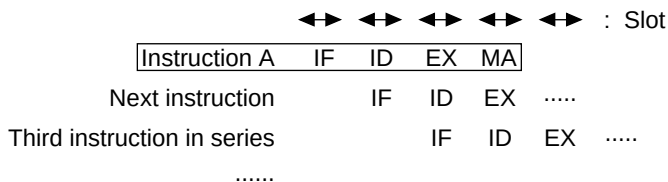
Figure 7.21 Memory Store Instructions Pipeline
