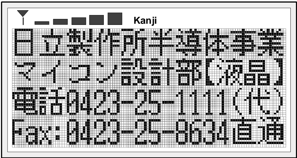
Figure 52 Example of Kanji Display in the Character Display Mode ( GR = 0 )
