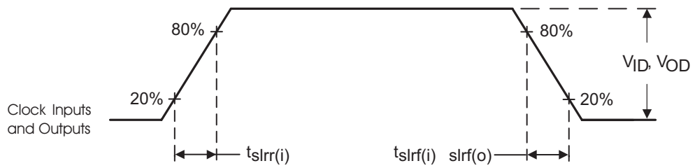
Figure 8. Input and Output Slew Rates
