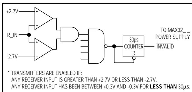
Figure 3b. MAX3221/MAX3223 with Transmitters Enabled Using AutoShutdown
