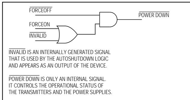
Figure 3c. AutoShutdown Logic
