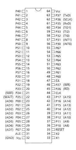
Figure 2.1 (1). Pin Assignment (Shrink Dual Inline Package)
