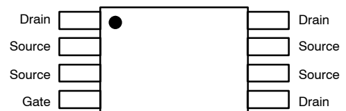
Figure 2. Pinouts for Single Die TSSOP
