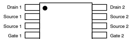
Figure 3. Pinouts for Dual-Die TSSOP
