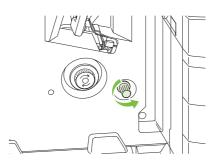
6. The jam-release knob is the larger, green dial on the left. Push in the jam-release knob, and then turn it clockwise to move any jammed paper into the output bin.
