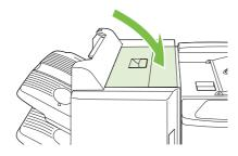
4. Lift the swing guide panel in the output bin. If you can see any jammed paper, gently pull it out.
