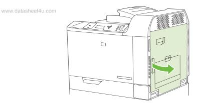
2. Lift the green handle on the transfer-access panel and open the panel.
