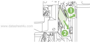
3. Grasp the blue handle for the stapler carriage and pull it straight out.
