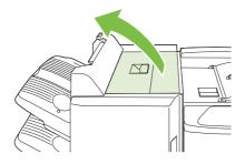
2. Remove jammed paper from the output bin or from the inside of the finishing device.
