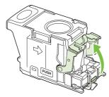
4. Remove the damaged staples that protrude from the staple cartridge. Remove the entire sheet of staples that the damaged staples were attached to.
