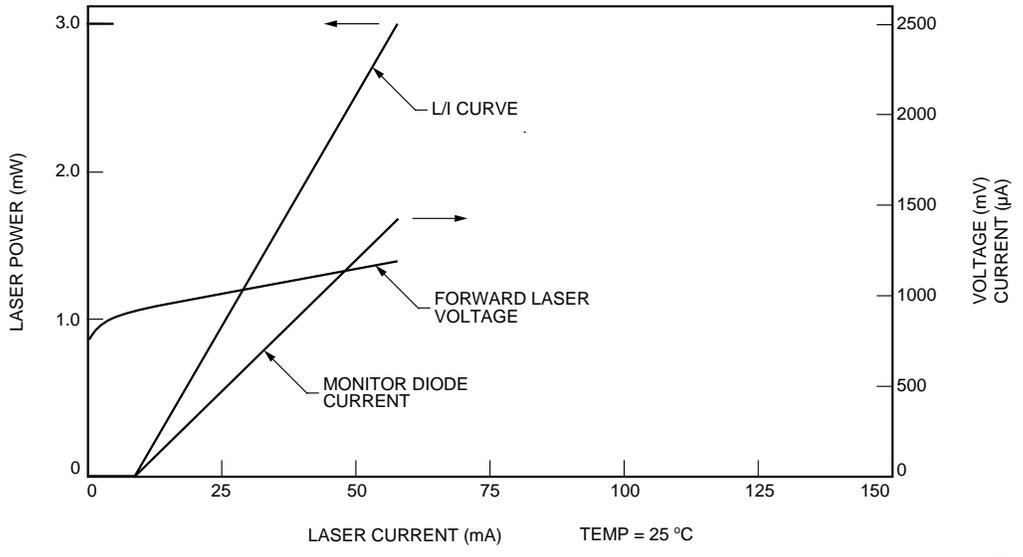
Figure 2. Typical D370-Type Laser Module L/I Curve
