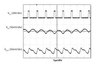
Waveforms During Over-Voltage Protection
