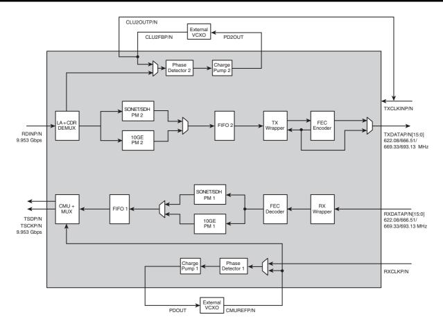
The BCM8512 is an 10 Gigabit DWDM transport processor that supports all the major functions on a DWDM line card:
